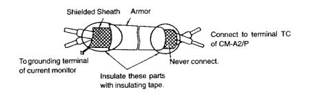
Fig. 4 Shielded wire termination
