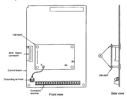
Fig. 2 Installation of current monitor card CM-A2/P
